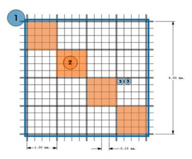
Fig. 1: Layout of a Fuchs Rosenthal Counting chamber
